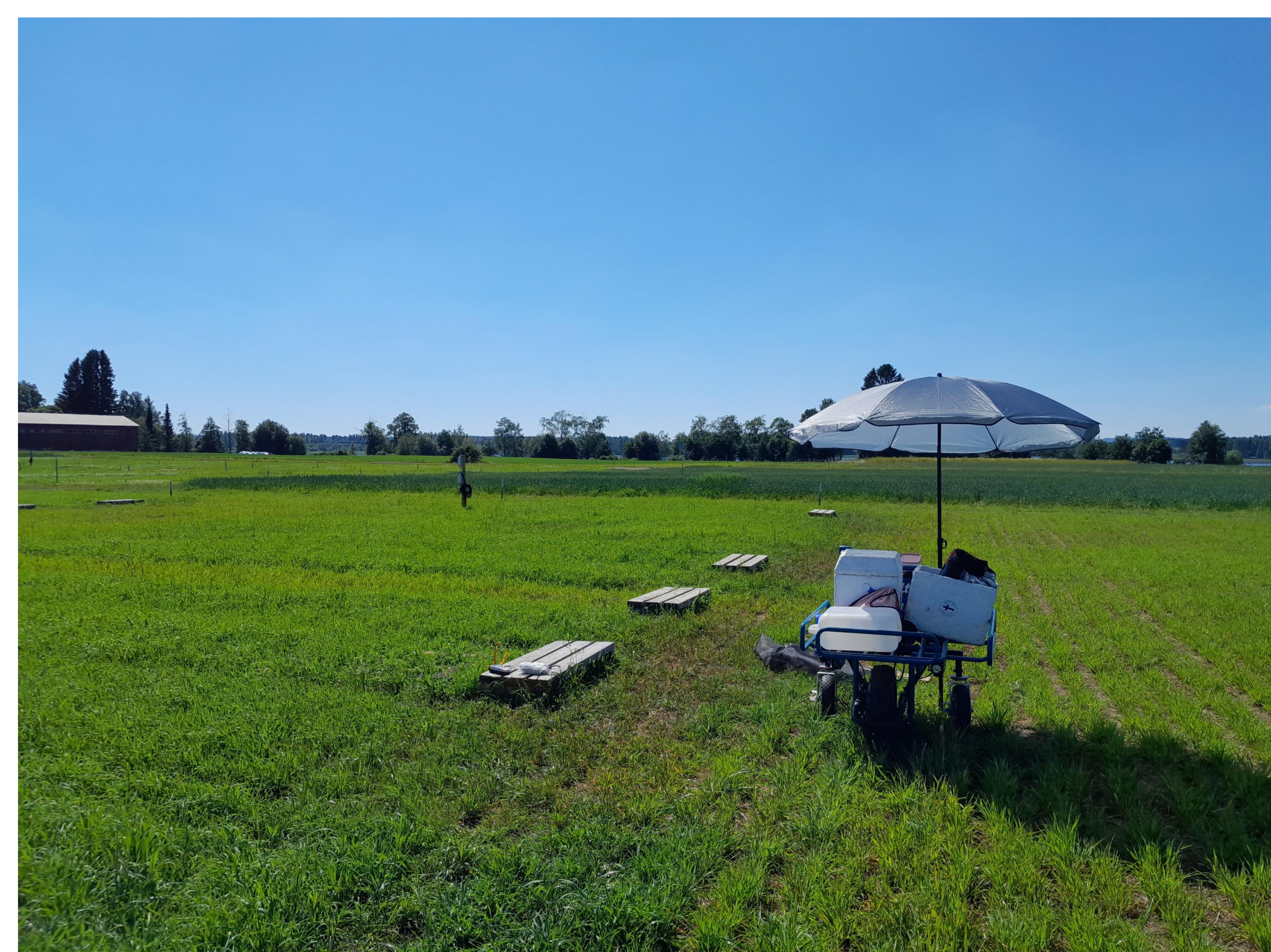
Figure 2. N 2 O fluxes were measured with closed chamber method with portable analyzer (LI-7820) in snow-free periods and with the snow gradient method during snow-cover.
