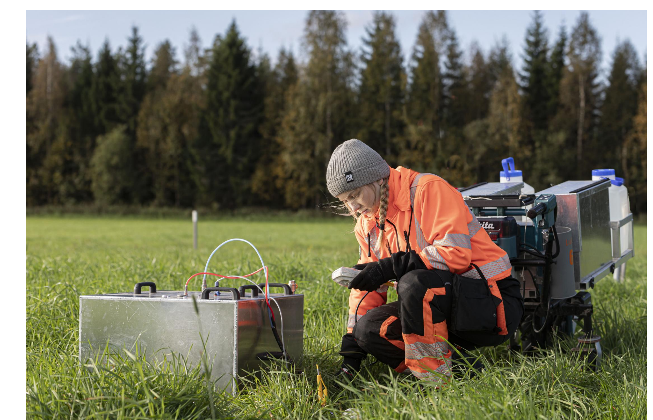
Figure 2. Closed chamber method with a portable analyzer was used for measuring N 2 O emissions during snow-free period.
