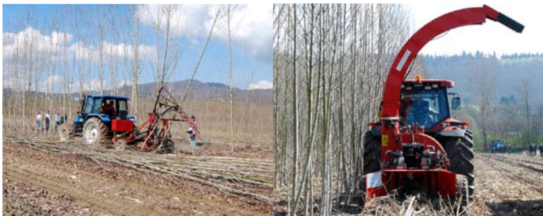
The Italian company Spapperi has developed harvest technology for small and medium scale poplar plantations. The trees are first cut down (on the left) and subsequently are chipped and blown into a transport trailer (on the right). (Photo: L. Corbella & M. Cocchi, ETA)
