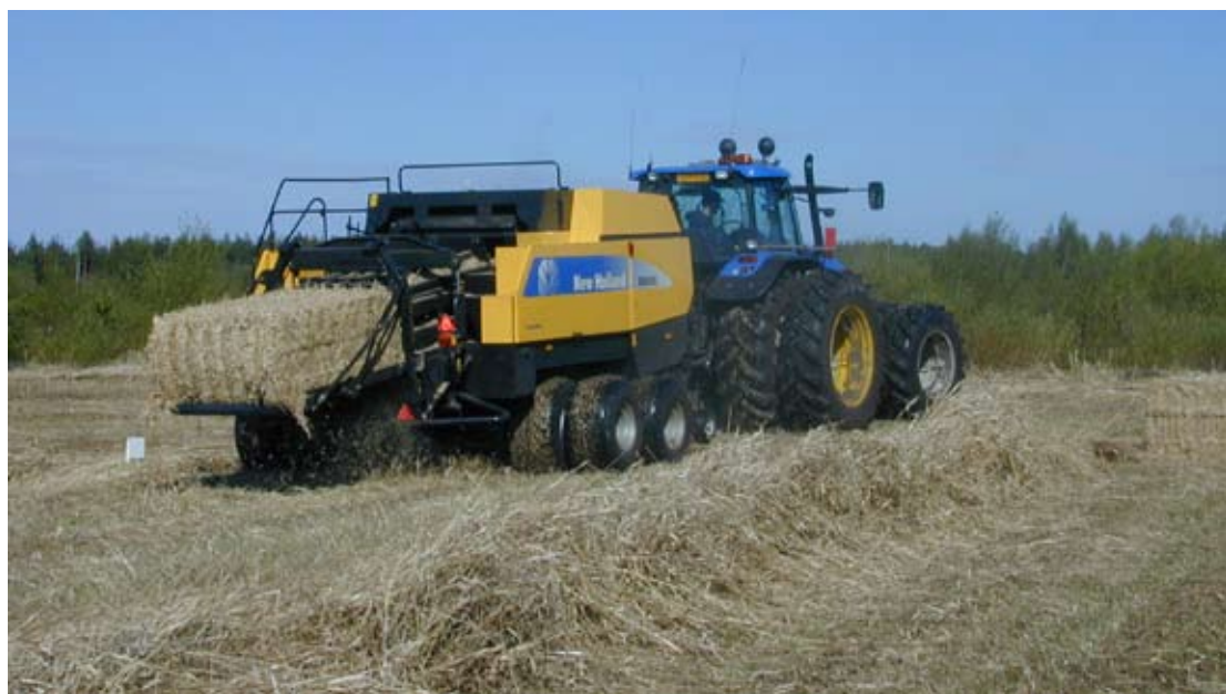
Advantages of a large square baler are the tight and well-shaped bales. (Photo: Timo Lötjönen, MTT)
