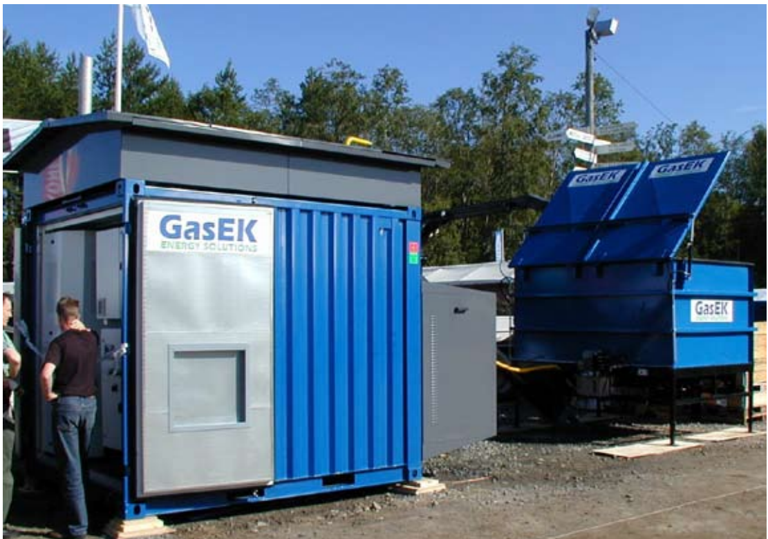
The GasEK small scale CHP-plant is a brand new Finnish innovation, which can gasify wood chips of under 40% moisture content. Total output of the plant is 90 or 150 kW, which includes about 33% electricity. (Photo: Timo Lötjönen, MTT)
