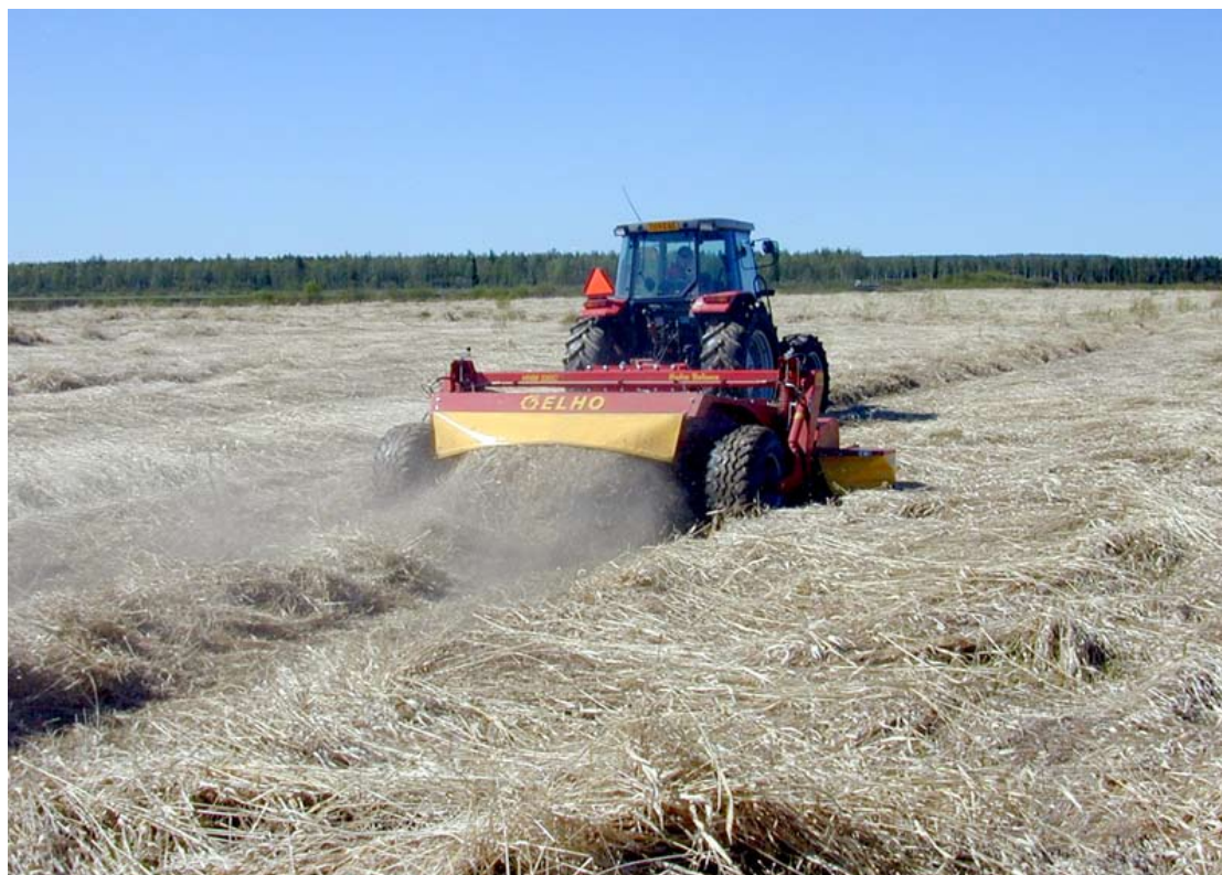
Disc mower with conditioner mowing RCG in spring. The snow has pressed the crop very near to the soil surface and it is therefore important to set stubble height as short as possible. (Photo: Timo Lötjönen, MTT)
