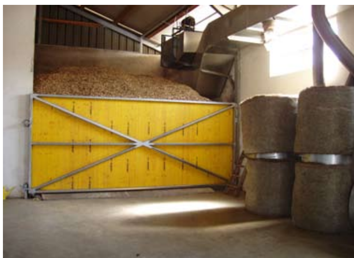
In the center box for drying wood chips; on the right - facility for drying hay. (photo: IEA Tulln, Gabauer)
