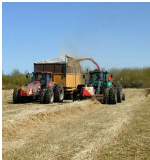
RCG can also be harvested as a chop, when it is easy to mix with main fuel at fuel terminal or on the yard of a power plant. (Photo: Timo Lötjönen, MTT).
