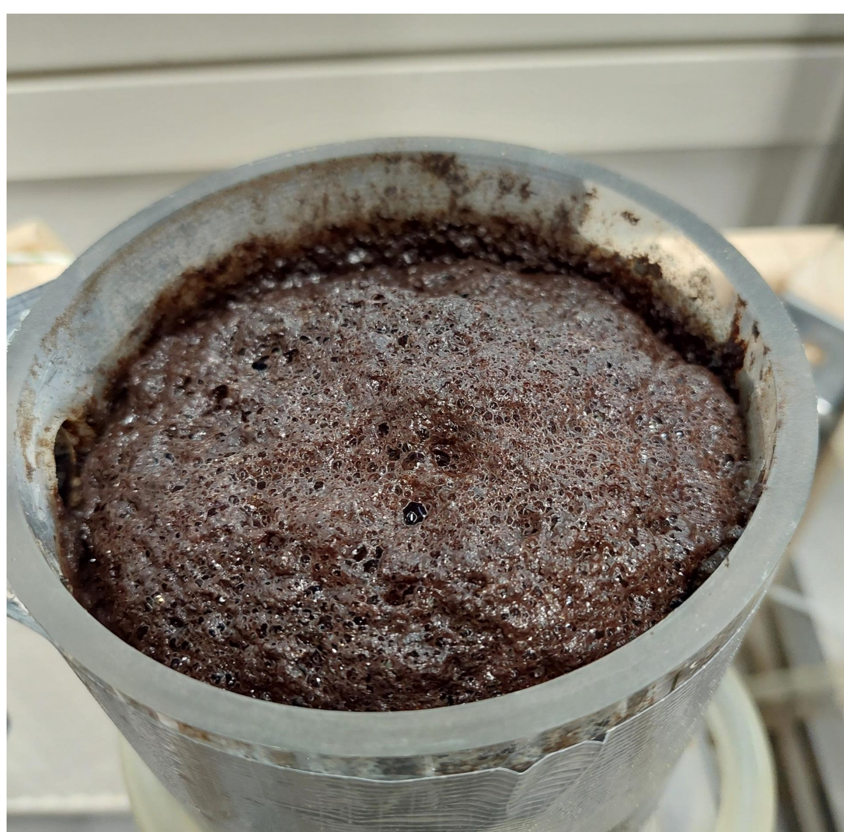
Figure 3. Flocculated solids disrupted the gas separation.
