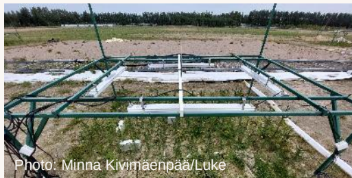
IR-heaters on the racks (target +5 °C in the picture)
